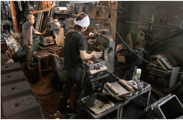
Dozens of jolt-squeezers making molds manually
