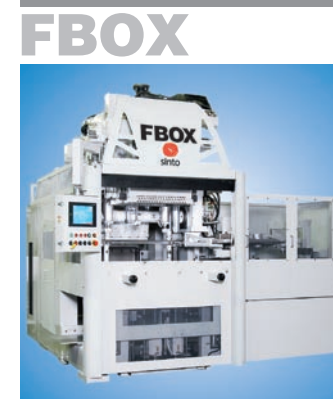
Flaskless molding machine (single station)
