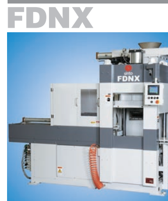
Flaskless molding machine (single station)
