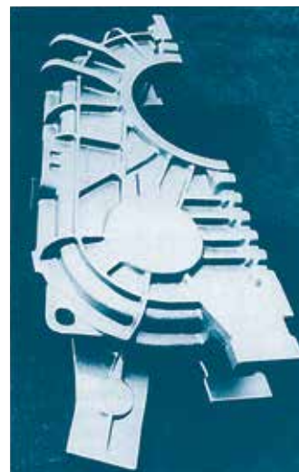
■ Picture 26: Gear box for the drive of a electric locomotive; Material: GGG-40, Mass: 200 kg
