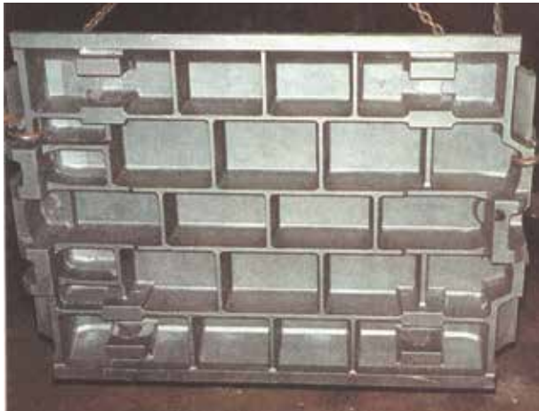
■ Pallet bogie for moulding machine; material: GJS-500-7, mass: 1070 kg, dimensions: 1800 x 1200 x 160 mm
