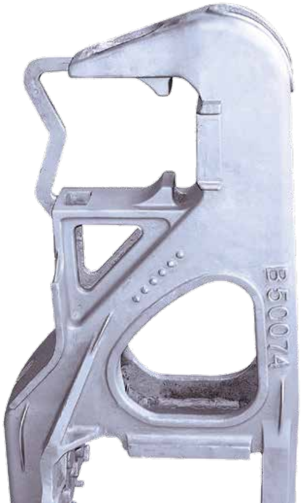
■ Railway chassis-frame material: Carbon steel, mass: 430 kg China
