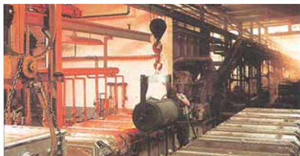
■ Picture 8: Pouring of vacuum moulds with vertical mould joint
