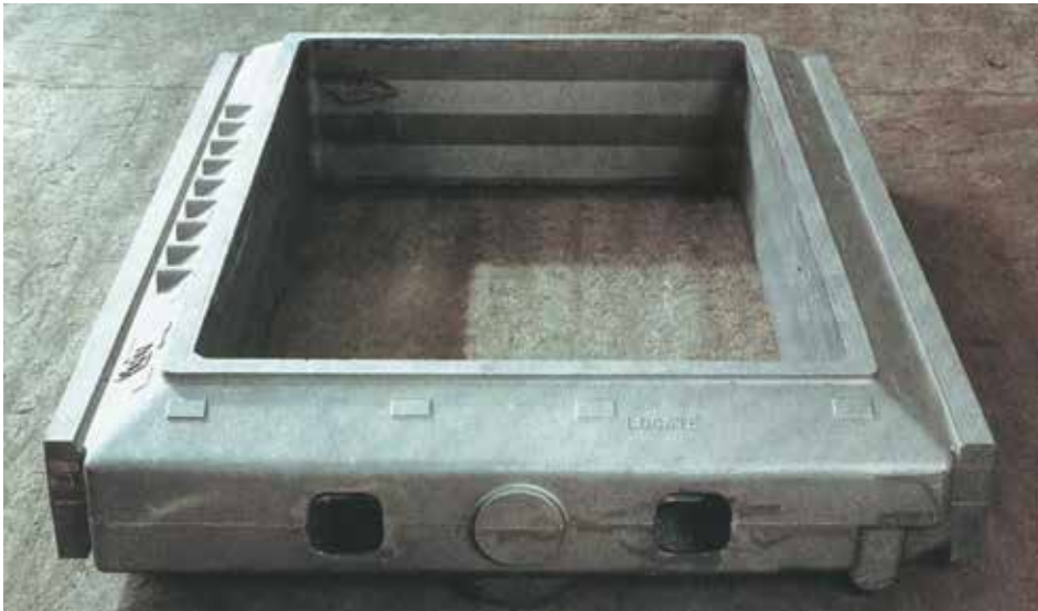
■ Moulding box for a moulding machine; material: GJS-500-7, mass: 800 kg, dimensions: 1790 x 1400 x 350 mm
