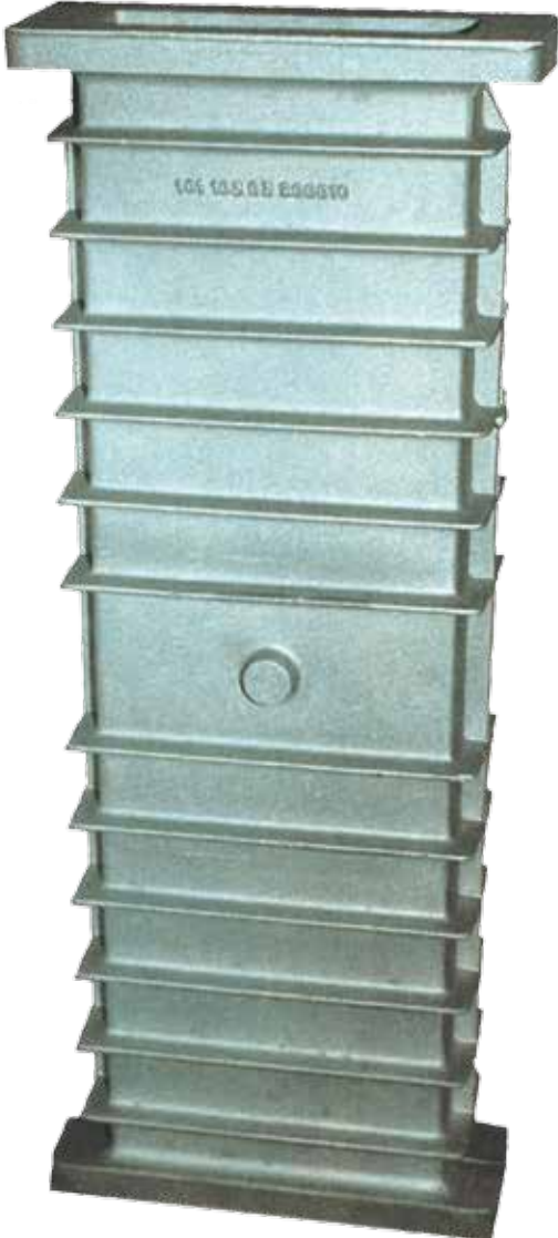
■ Cooler case with high demands to the gas tightness, material: G-AISI10Mg wa, mass: 10 kg, dimensions: 710 x 300 x 120 mm
