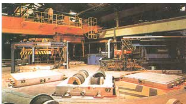
■ Picture 3: Part of a vacuum moulding plant with horizontal mould joint (core setting line)
