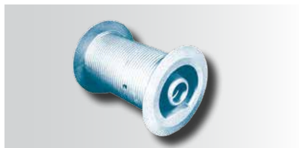
■ Picture 11: Rope drum; material: GGG-40 or GGG-40.3, dimensions: 790 x \varnothing 650 mm, Mass: 280 kg; dimensional evaluation of 15 castings see table 2
