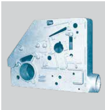
■ Picture 17: Side flask; material: G-AlSi8Cu3, dimensions: 650 x 480 x 130 mm, mass: 11 kg
