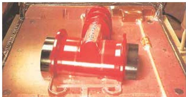
■ Picture 5: Pattern with film sucked accurately to the shape by vacuum
