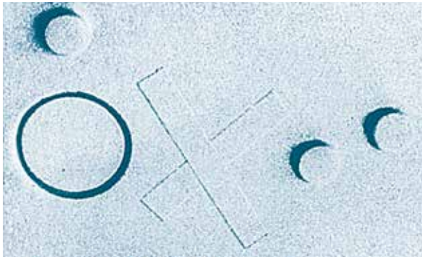
■ Picture 20: The crack of the pattern film was repaired with scotch tape – an accurate detail revealed by applying the vacuum process
