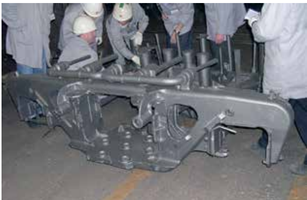
■ Railway chassis-frame type 4 material: Carbon steel Russia
