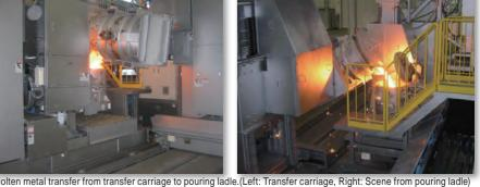
Molten metal is transferred from the transfer carriage into the pouring ladle.
