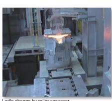
Molten metal is transferred by exchanging ladles between transfer carrier and pouring machine. This method prevents temperature drop of molten metal and is good for reduction of casting defects.
